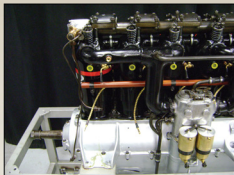
Water jacketed intake manifold and carburetor detail. A mount for the generator (E4) can be seen at right but the actual generator was very rarely installed in fighter aircraft.
