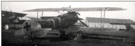
This ex. Jasta 23b Roland D.VIa was handed over to the allies after the armistice and is pictured here at Koblenz. Note that the guns had been removed by the time this photo was taken. Other photos of this aircraft show it to have the early 160hp Daimler-Mercedes D.III engine installed. The dark band around the fuselage appears lighter than the black Jasta 23b fuselage markings which could indicate that it was a different colour, red perhaps? (Greg VanWyngarden)
