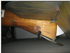
Tailskid fairing and bungee cord details. The horizontal tailplane is a single piece which slides through the rear of the fuselage.
