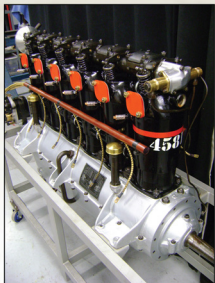
The serial number of the engine was sometimes stenciled on the front of the cylinder and the red band signifies an over compressed engine, both colourful touches seldom seen in archive photos.
