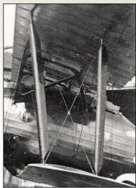
Early style struts as seen on the 1st few Roland D.VI, in this case from Otto Kissenberth's D.VIa.
