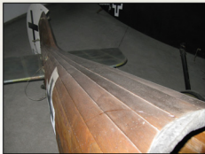
Fuselage spine showing the unique Roland overlapping plank on plank construction detail.
