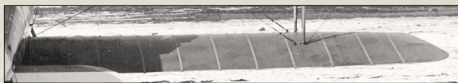
Lower wing details from the Jasta 23b Roland D.VIa from page 13 showing the rigging attachment points, 4 colour lozenge fabric covering and unpainted linen rib and edging tapes. (Greg VanWyngarden)
