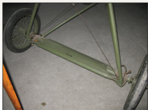
Undercarriage axle wing from Roland D.VIb 2225/18 showing the grey-green colour of the wooden struts and hinged metal axle flap. Note how the rigging attaches to the axle wing. (Krakow Museum Poland)
