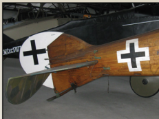
Rear of fuselage showing lifting hand holes and control cable outlets. Note that rib tapes were not applied to the elevators of Great War era Roland D.VI aircraft.
