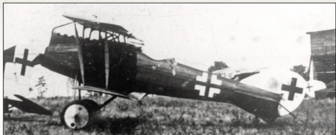
This unidentified Roland D.VIa features a dark fuselage, late style struts and an early 160hp Daimler-Mercedes D.III engine. A painted over personal marking appears just forward of the fuselage cross and the fin has been painted white, interestingly this does not follow the outline of the front of the fin. The shoulder straps of the pilot's four point harness can be seen hanging over the edge of the cockpit opening.
