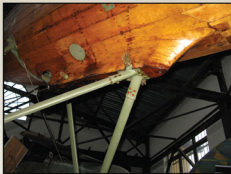
The rear undercarriage struts meet under the fuselage. Note the lower wing attachment lugs.
