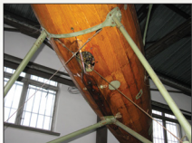
Undercarriage strut detail from Roland D.VIb 2225/18 showing the grey-green colour of the struts and various metal fuselage fittings. Note how the rigging enters the fuselage. (Krakow Museum Poland)
