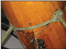
Front undercarriage strut attachments showing wire threaded through the bolts to prevent them working loose in service. Note the drain hole.
