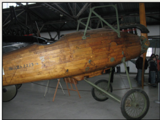
Forward fuselage showing various brackets and strut attachment details.
