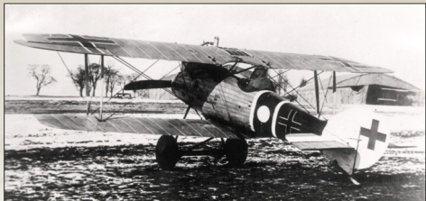
This photo of a Jasta 23b Roland D.VIa shows the same aircraft at Koblenz as option E but at a later date. There is a white circle painted on each side of the fuselage and the wheel covers have been painted black (or another dark colour). For other views of this aircraft see pages 13, 26 and 29. Note the position of the Roland factory decal below the rear of the cockpit opening. (Greg VanWyngarden)
