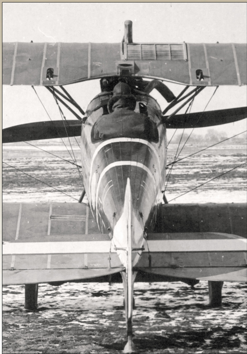
Close up view of the unarmed Jasta 23b Roland D.VIIa shown on page 13. Details to note include the overlapping planking along the fuselage spine, serial number stencil on tailplane (unfortunately not legible) and the brackets on the right side of the fuselage to support a spirit level on the datum line during assembly. (Greg VanWyngarden)
