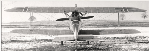
A nice rear view of the same Jasta 23b Roland D.VIa seen above. This aircraft was handed over to the allies after the Armistice and is shown here undergoing trials at Koblenz. It's colour scheme closely resembles our option E but with a small white circle in the dark fuselage band and dark wheel covers. Note how the tailplane is out of alignment with the lower wings. (Greg VanWynyarden)
